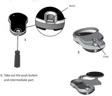
c. Take out the electronic board with the battery and remove battery.
