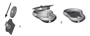
Reassemble the intermediate part and the push button and place over the electronic board.
