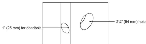
**Note:** drill 2 $\frac{1}{8}$ " (54 mm) hole from both sides of the door to avoid damaging the door
