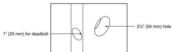
**Note:** drill 2 1/4" (54 mm) hole from both sides of the door to avoid damaging the door
